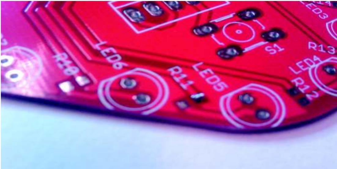
2. Heat up the solder on the pad and place the resistor on top using the tweezers. Then remove the soldering iron while holding the resistor in place. Let go of the resistor once the solder has cooled (does not take long).
