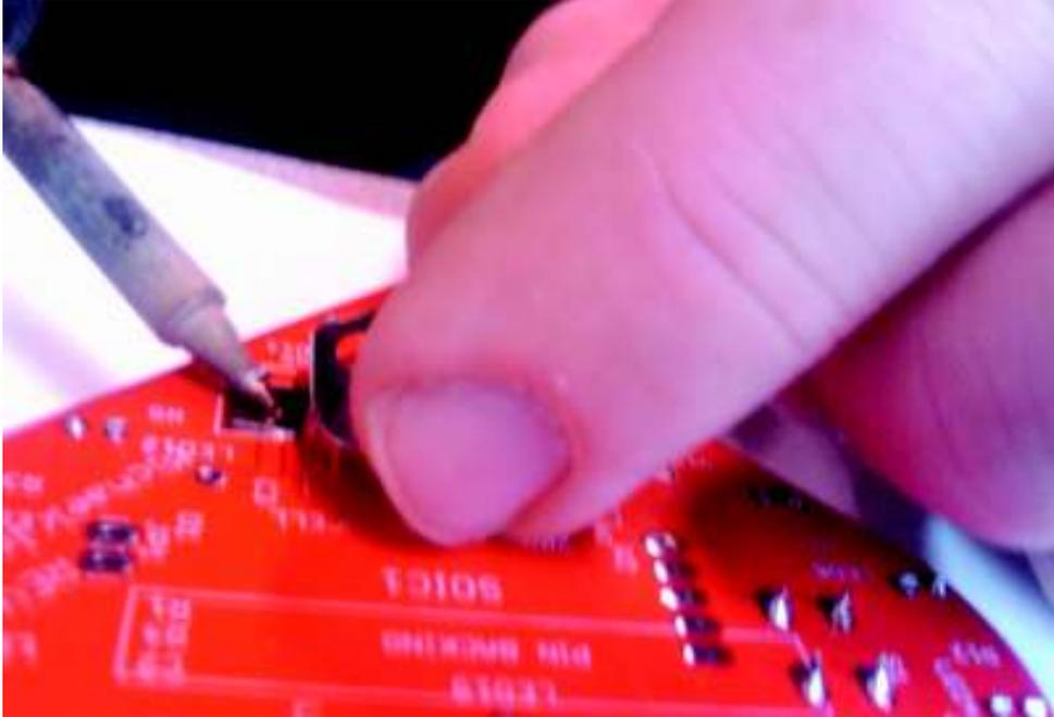
4. Add solder to the other pad to attach the other side of the battery holder.
